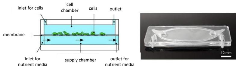
At KIT, the Institute of Microstructure Technology in cooperation with the Botanical Institute has developed a microfluidic bioreactor in which plant cells can be cultivated. Its modular design allows to connect different cell types with each other by a common metabolic flow and thus to generate new substances or to increase efficiency, if necessary.
